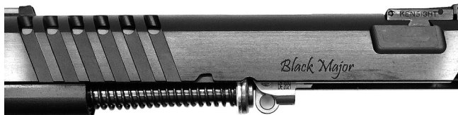
Figure 7.7: Slide with barrel, barrel link and recoil spring assembly
